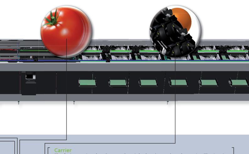
The fruits are singulated, rotated, weighed and sorted on the carrier. The 3-point weighing system guarantees precision, even at high speeds.
